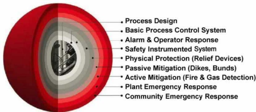
Figure 4: Layers of Protection
